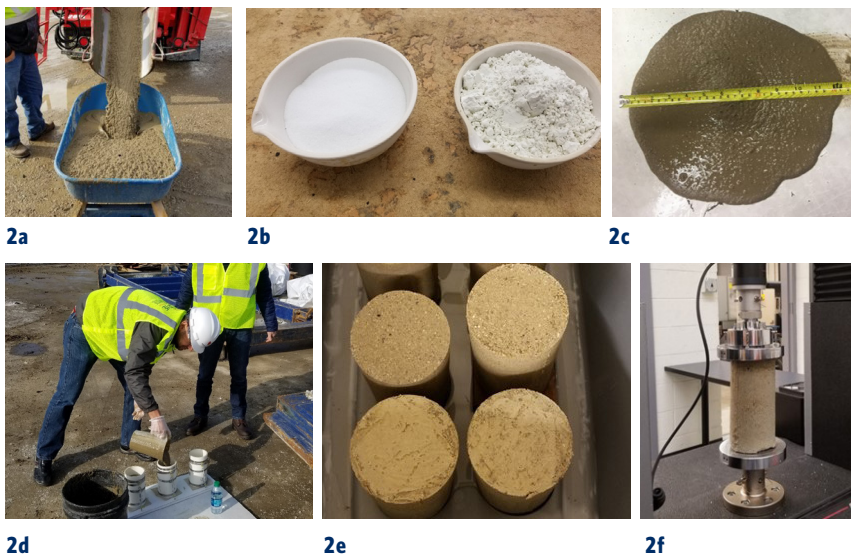
FIGURE 2. Students making and testing flowable fills samples with cleaned and grounded waste glass powder (a) application of flowable fill in the field; (b) cleaned and grounded waste glass powder coarse (left) and fine (right); (c) flow test; (d) making flowable fill specimen for strength test; (e) dried flowable fill specimen for strength test; (f) strength test
