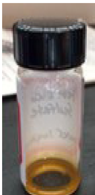
FIGURE 4. Water sensitivity of ferrous sulfate is measured. Distilled water (0.5 mL) was added to ferrous sulfate (0.1 g).
