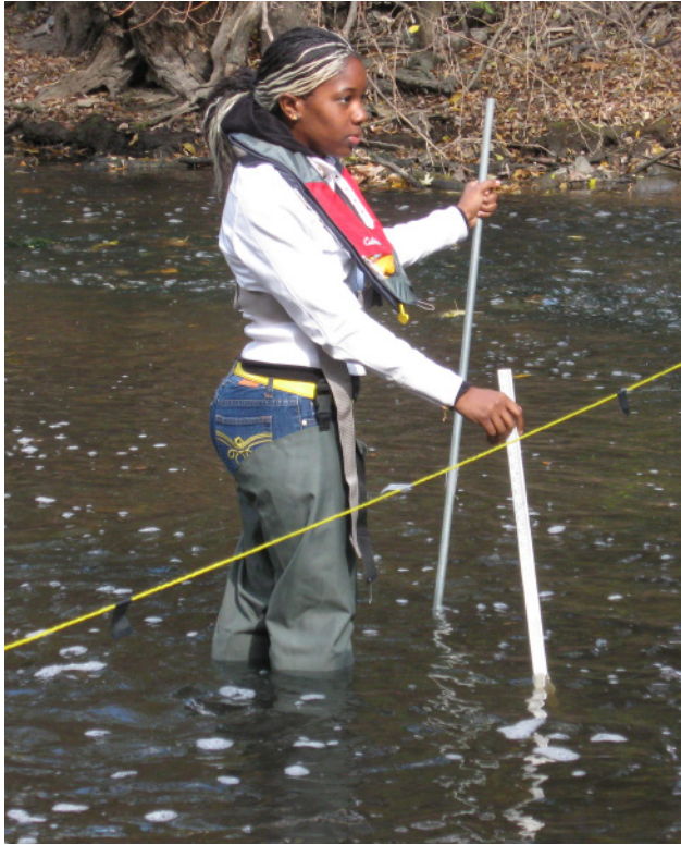
FIGURE 1. Student measuring stream discharge in the North Branch of the Chicago River .
